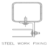
STEEL WORK FIXING
