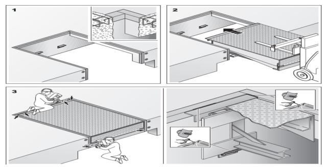
If pit mounted, angles cap off the concrete to form the edge of the pit on all 6 sides (5 sides if suspended frame as shown above). With this design, the dock leveller is simply lifted into the pit, shimmed and levelled to suit the surrounding floor level, bolted to the concrete base or welded if steel and welded across the full width of the rear hinge angle.
