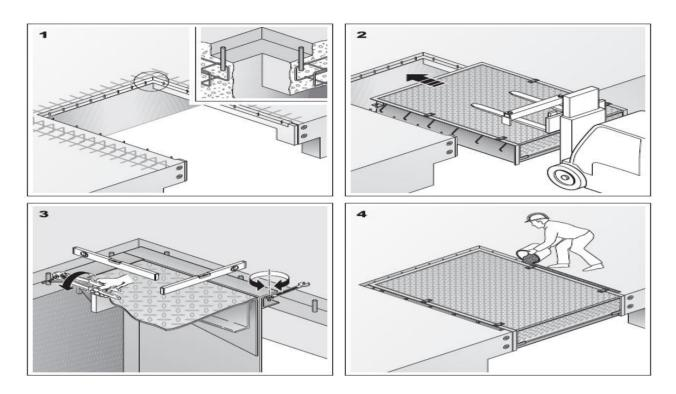
The second suspended frame design does not require a pit edge angle set. The pit is cast leaving a 100mm deep x 150mm rebate around the edge of the pit. The pit will have a series of reinforcement pins placed around it. The dock leveller is lifted into place, shimmed and levelled to the finished floor level. The dock leveller frame tangs are then welded to the pins. The customer then infill's the rebate to finish the mechanical installation.
