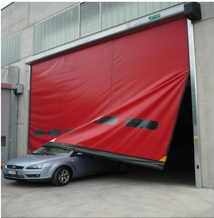
This large Delta Speed 7500 demonstrates the ability of the curtain to withstand impact from vehicle traffic. The next opening cycle will self repair the curtain and the door will automatically close ready for use. No tools needed and automatically
